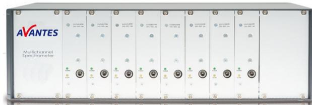
Multi-channel spectrometer with 10 channel configuration
