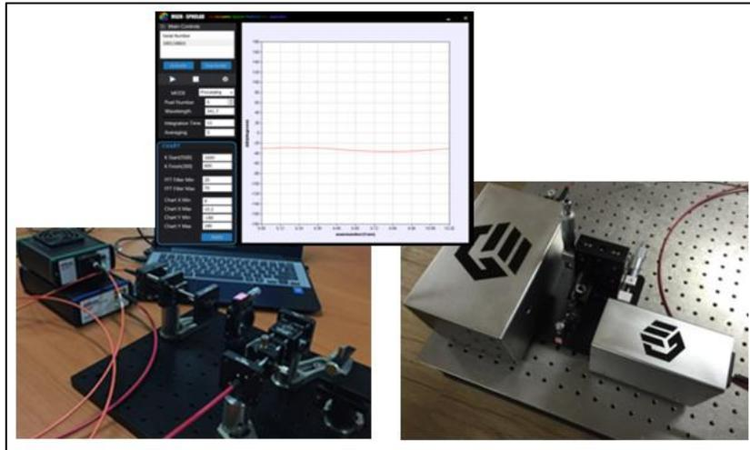
AvaSpec and AvaLight have been used to get highly accurate and stable spectra in real time speed. Thanks to the stability of these components we were able to achieve the  $\Delta(k)$  measurement repeatability of around  $0.1^\circ$  with the measurement speed of 20Hz. To our knowledge, this is the first dynamic  $\Delta(k)$  measurement demonstration in the spectro-polarimetry and ellipsometry.
