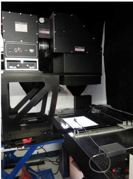
AvaSpec-SolarXM measuring solar simulator
