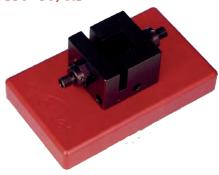
The CUV-UV/VIS, CUV-FL-UV/VIS and CUV-ALL/UV/VIS are especially designed for absorption and fluorescence measurements and should be used with standard 10x10 mm cuvettes. For non-standard cuvettes, adjustable ball-detents ensure repeatable placement and measurements at the same location. All cuvette holders have a 5 mm wide slit to hold filters and a cover to prevent ambient light from entering the light path.
