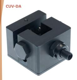
To mount a cuvette holder directly to your light source, Avantes offers a range of direct-attached cuvette holders. The CUV-DA connects to the AvaLight-DHc, -XE and -(HP) LED light sources, the CUV-DA-DHS to the AvaLight-DHS and AvaLight-DHS-BAL and the CUV-DA-HAL to the AvaLight-HAL. These devices can be used for either absorbance or fluorescence measurements.
