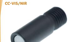
To collect light from a 180° angle, cosine correctors are used. This eliminates optical interface problems associated with the light collection sampling geometry inherent to other sampling devices such as bare fiber-optics, collimating lenses or integrating spheres.
