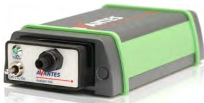
From visible light to near infrared, that's where the AvaLight-HAL-S-Mini works best. It's a compact, stabilized halogen light source, with adjustable focusing of the fiber connection, maximizing output power at the desired wavelength. The light source also has adjustable output power to provide extra power or longer bulb life.
