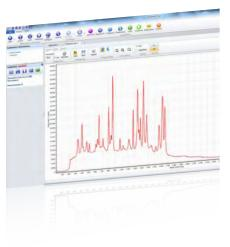
For online and offline reflective color measurements, AvaSoft-COL is the ideal companion. This application provides a precise way to perform color measurements using the basic principles and techniques defined by the International Commission on Illumination (CIE). The CIE 1976 L\*a\*b\* color parameters are calculated, along with other parameters, like Hue, Chroma and X, Y, Z.
