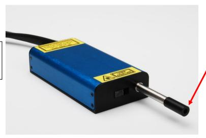
Attach Distance Regulator for Solid Samples
