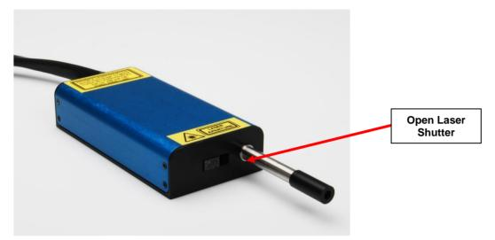
7. Place solid sample in contact with the distance regulator, or if using a liquid sample position the sample in front of the probe and adjust the position so that the liquid is ~9mm from the end of the probe shaft (without distance regulator).
