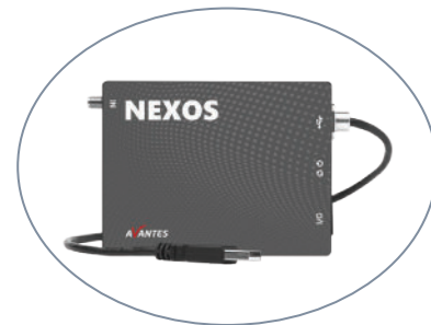
AvaSpec-NEXOS™ 2048 and 4096 pixel options 190-1100 nm
