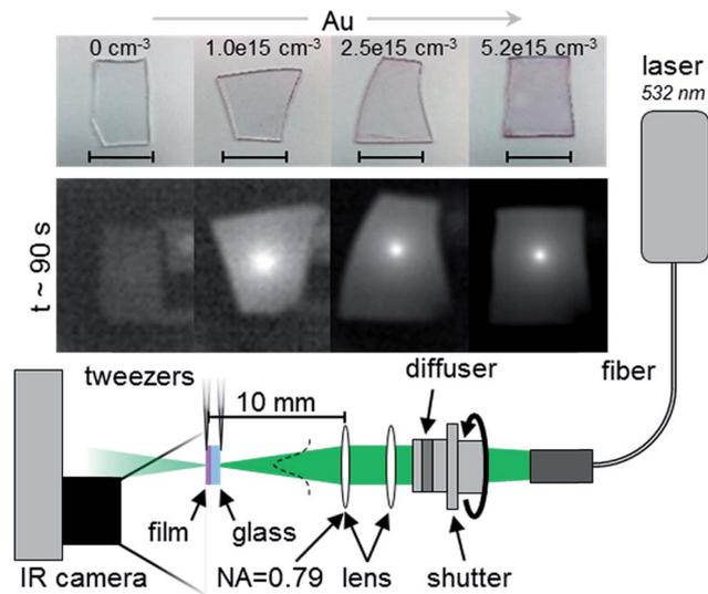
**Scheme 1** Apparatus for thermal characterization of AuNP–PVP films shown in optical images (top row) and in infrared images captured at steady-state after approximately 90 seconds of irradiation (bottom row). Scale bar is equivalent to 1 cm. 10 mm scale bar in schematic is to indicate distance between focal point of last lens and focal point on sample. NA is the numerical aperture of the last lens.
