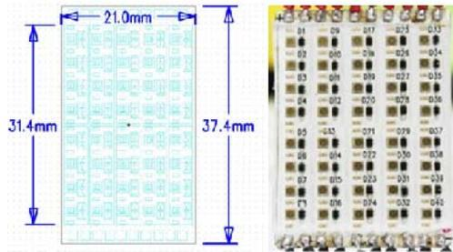
Fig. 1 Configuration of the prototype UV LED module
