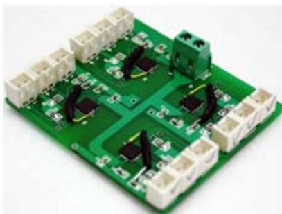
Fig. 2 The prototype UV LED driving circuit
