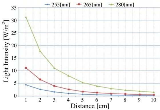
Fig. 5 Intensity of the UV LED modules
