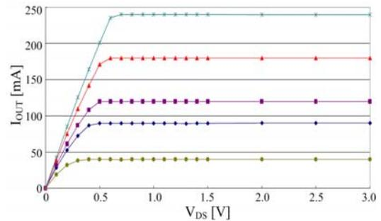
Fig. 3 Current characteristic of the driving circuit
