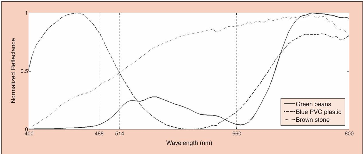
**Fig. 3.** The largest contrast between a green vegetable and the blue plastic is close to the 488 nm line; identification of the brown stone requires illumination with the 660 nm laser line.
