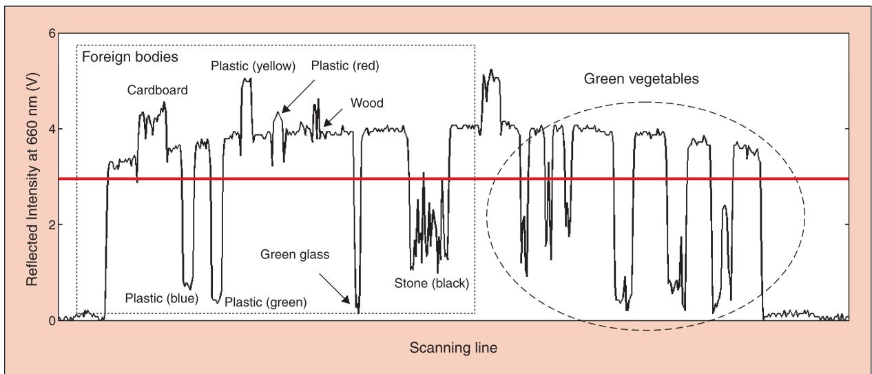
**Fig. 5.** Scan plot demonstrating the use of the reflected intensity at 660 nm as optical measure to separate non-green colored foreign bodies from green vegetables.
