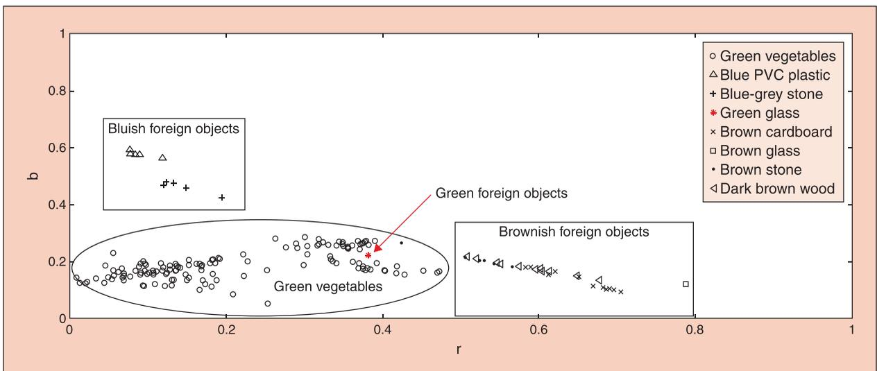
**Fig. 4.** Identification of bluish objects and brownish objects requires the use the two-color density parameters  $r$  and  $b$ .
