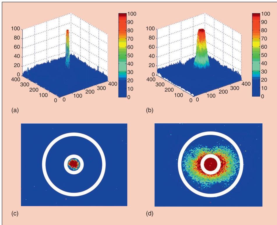
**Fig. 6.** Differences in scatter properties are distinct due to dissimilarities in porosity between (a) a piece of glass and (b) a potato. Simulation of the use of a ring sensor to separate light scattered in (c) the inner and (d) the outer parts of the scattered light beam.
